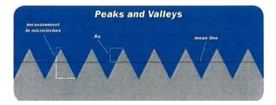
Ra - Roughness Average is an absolute average height whereby you establish a mean line and a number of height samples i.e. H1, H2, H3 etc. above and below the line
