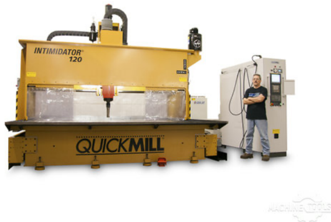
Figure 1 Roben's Quickmill Intimidator 120: High-power CNC machine with 120-inch travel.
